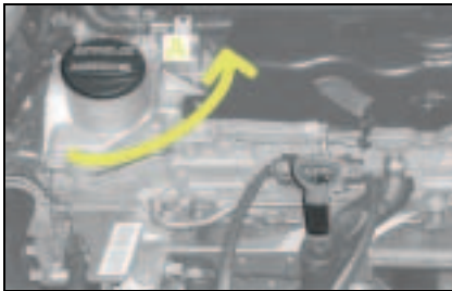
Oil filler hole, diesel engine
